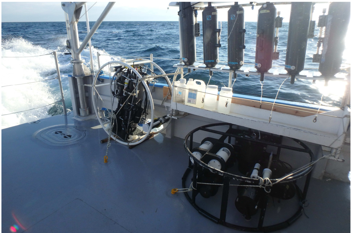
Niskin Bottles for water sampling and the two IOP packages for instruments intercomparison on the deck of the R/V Sagitta III.
